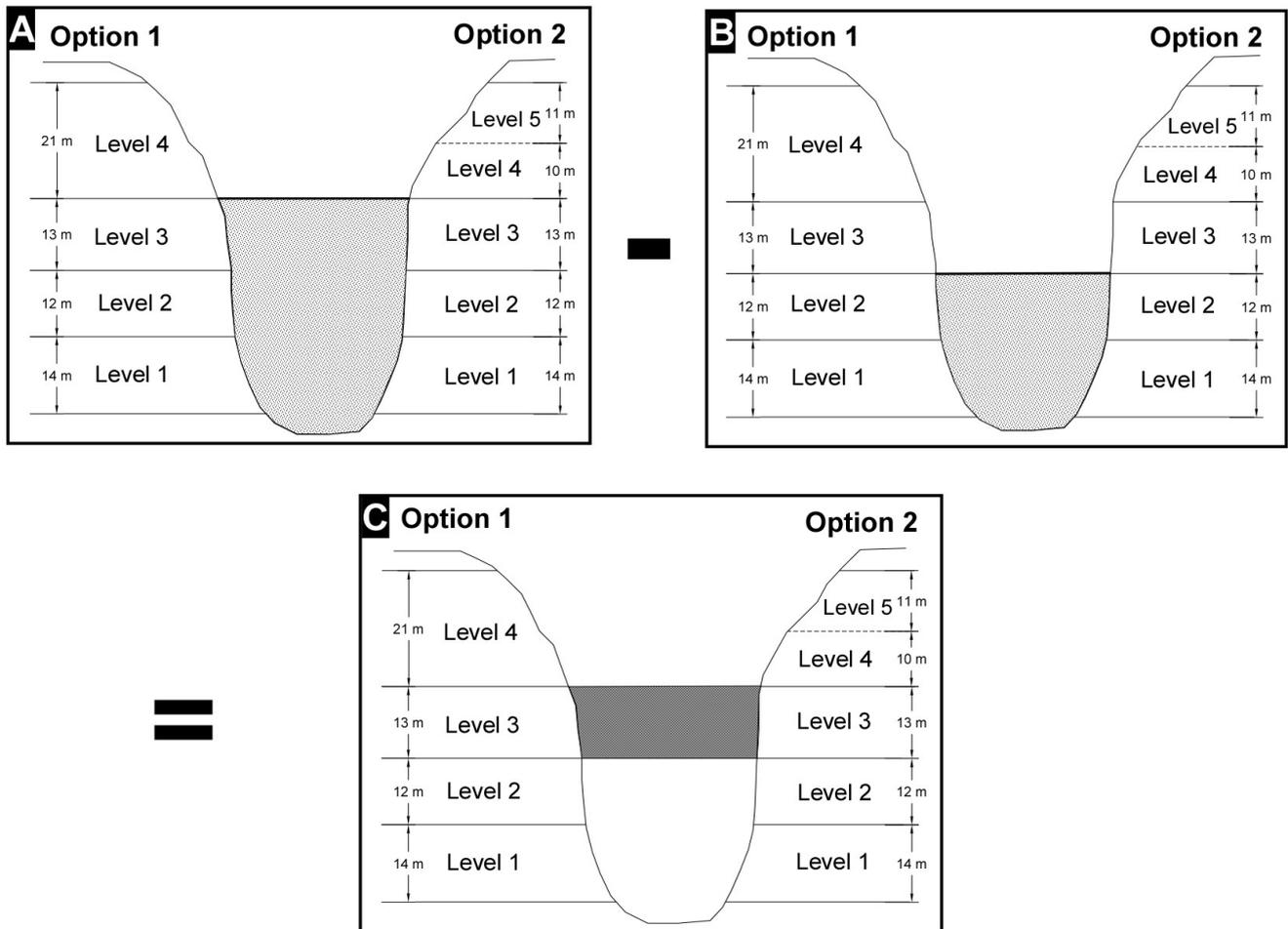
Figure 2. Visual depiction of how the 3D Analysis tool is used to calculate the volume of material removed and the surface area as represented for the study area. The GIS outputs the area and volume of the open space below a specified elevation (light gray, 2a and 2b). To find the area and volume for each level, 2a was subtracted from 2b, which gave the volume and area for each level (2c). Note that this figure is a schematic drawing and does not represent any specific location within the park.
